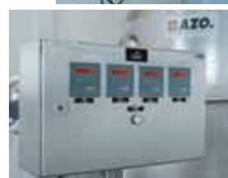
MCS operating terminal
