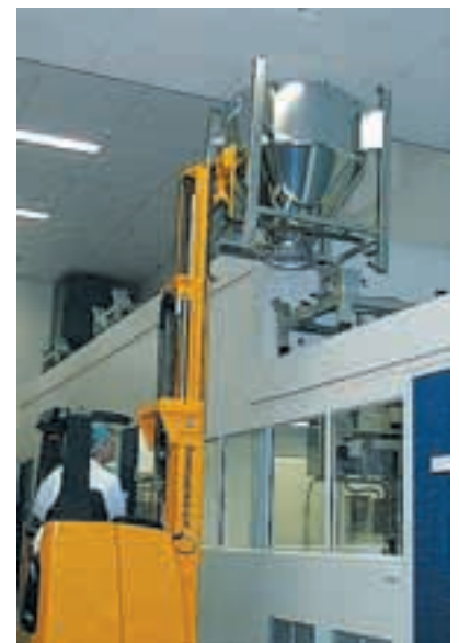
Interchangeable container over filling machine
