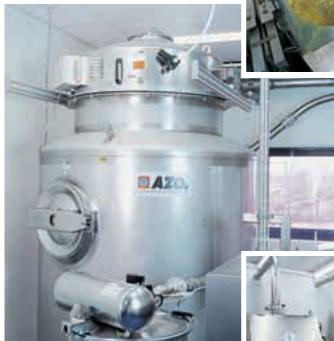
Filter with sliding arrangement for maintenance ease
