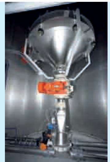
Dust free product intake and clean frame skirt through suction conveying: left – vibration bottom with dosing screw, right – with dosing rotary valve
