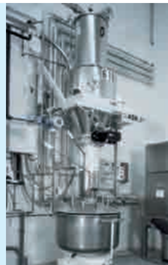
Feeding of kneading unit with a single pipe system
