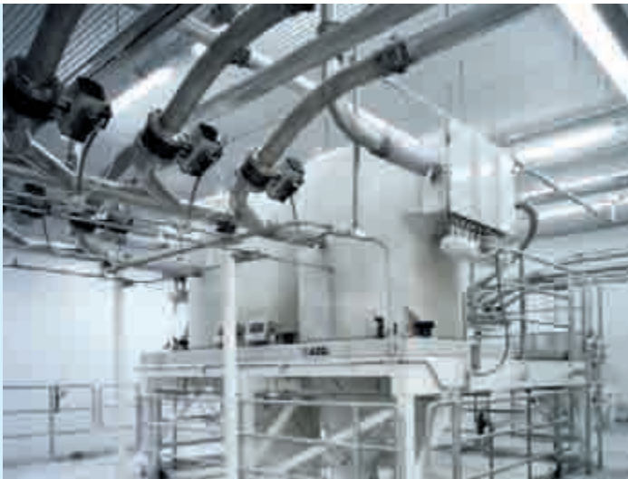
Several conveying lines lead to a common multi-port valve
