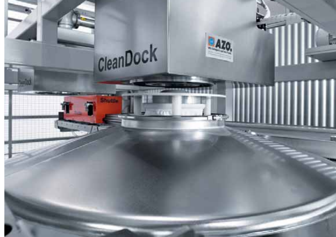
Docking a AZO®ShuttleTainer
