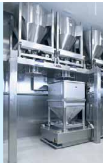
Linear arrangement of AZO DOSITAINERS®
