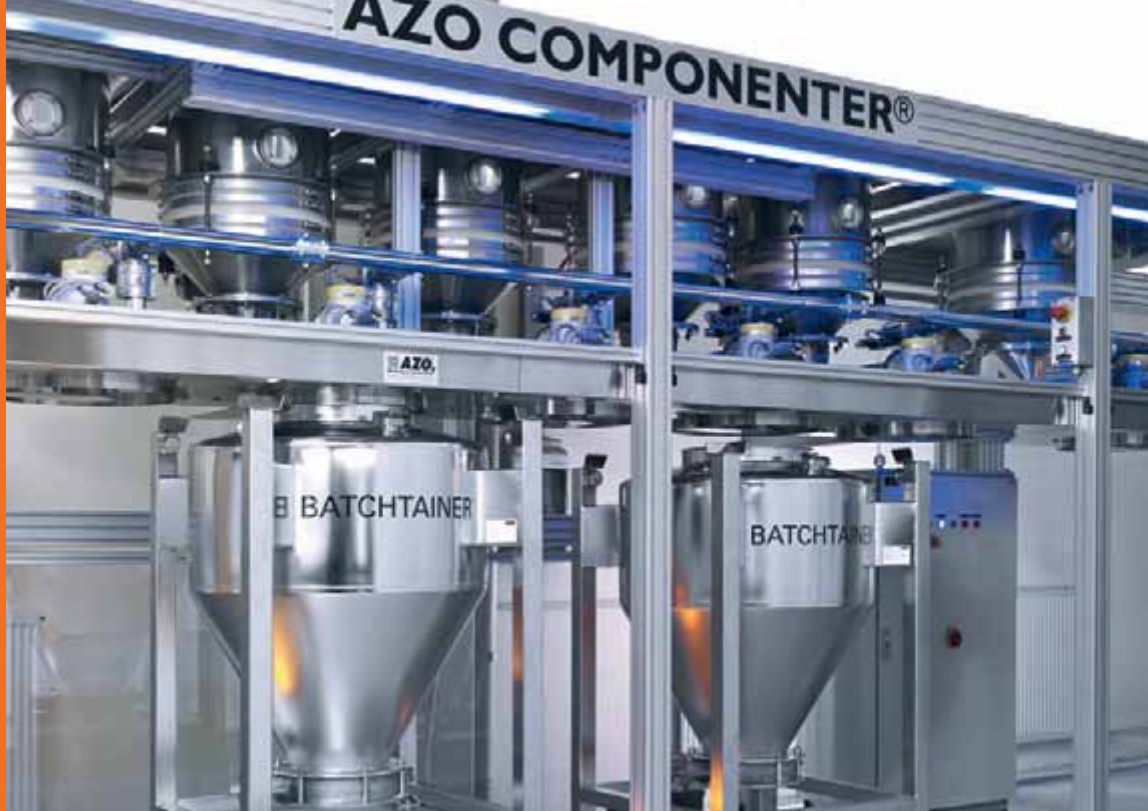
AZO BATCHTAINER® as collecting hopper
