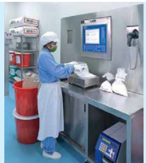
ManDos weighing station with barcode recording and label printer for weighing of active ingredients
