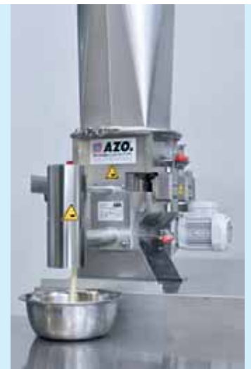
AZODOS® with micro-dosing system
