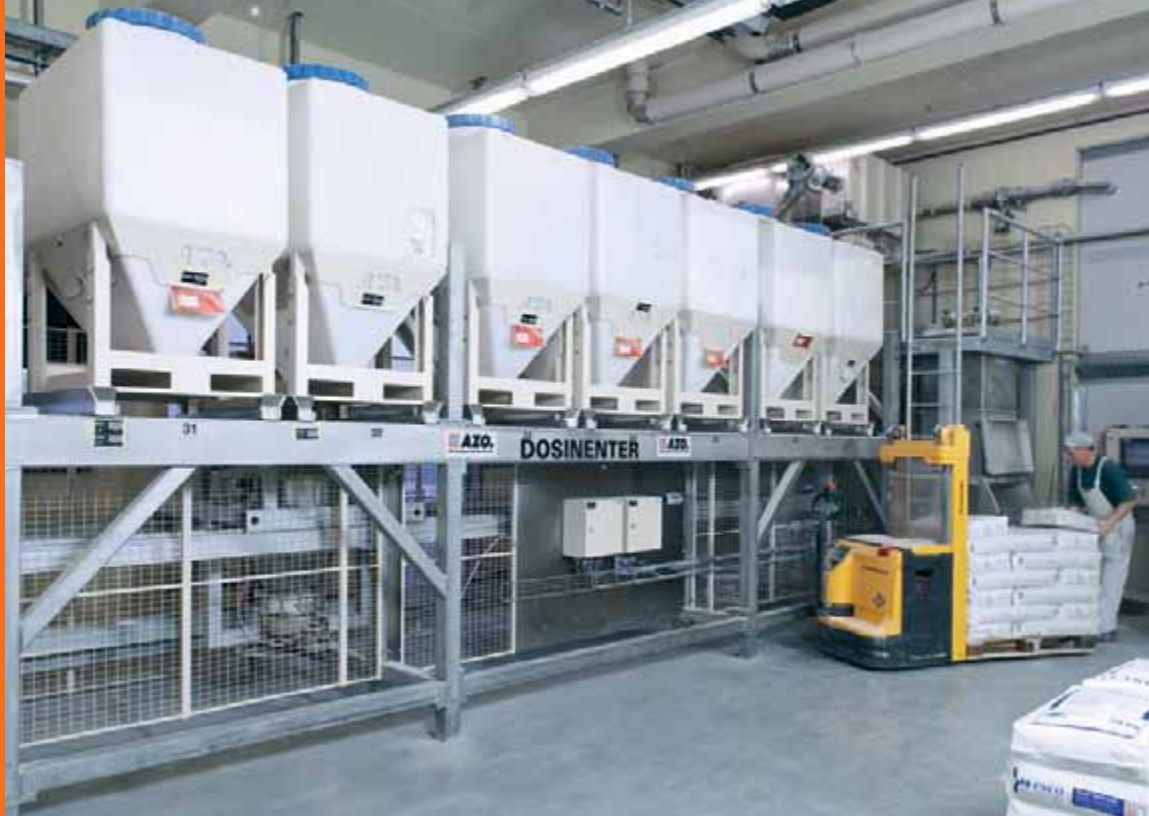
AZO DOSINENTER® in baking ingredient application
