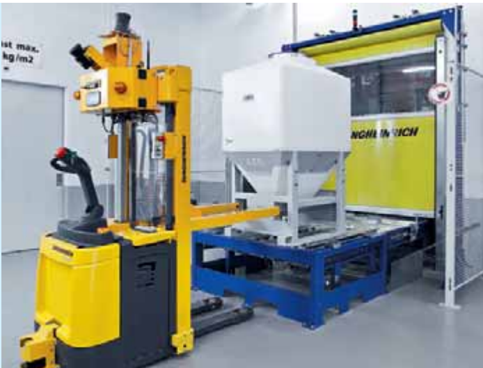
Storage and removal of DosiBoxes® with automated guided vehicles
