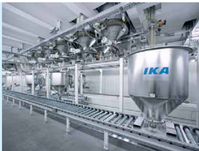
Collection of additives in an AZO MIXTAINER® with dynamic scales
