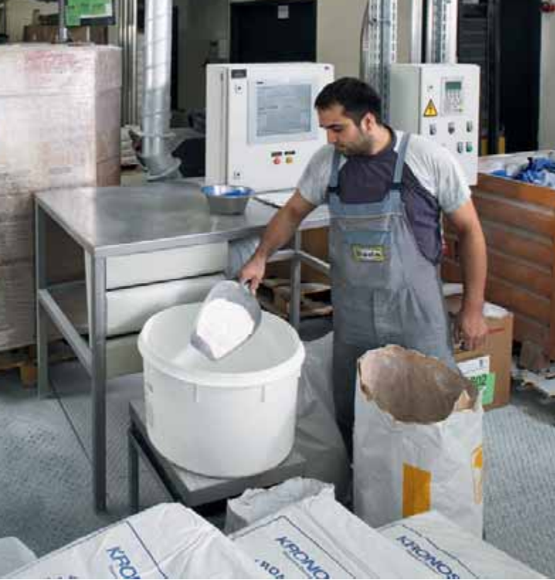
Manual weighing station for colours, additives and aggregates at a compound manufacturer
