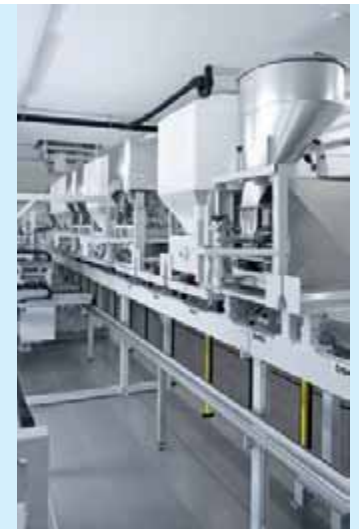
Foreground: micro-dosing module
