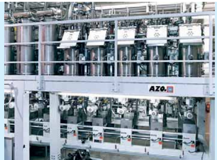
Feeding hopper and receiver can be used as surge bins
